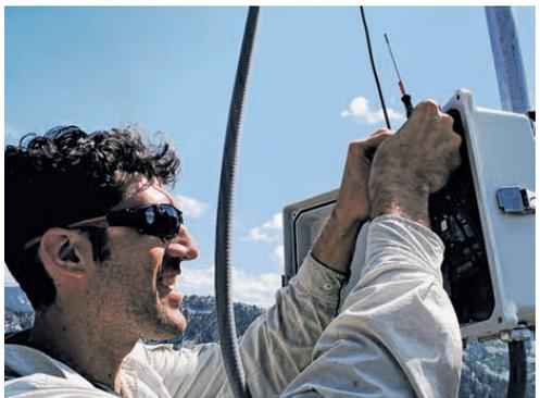
A Glaser team member checks out the sensor that will be attached to a 16-foot pole to help measure the state's water supply and beam the data to researchers.
